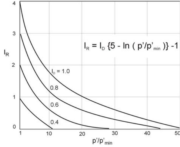
Fig. 2. The dependence  $I_R$  on  $p'/p'_{\min}$
