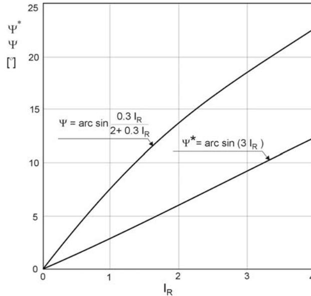
Fig. 4. The dilatancy angle as a function of  $I_R$
