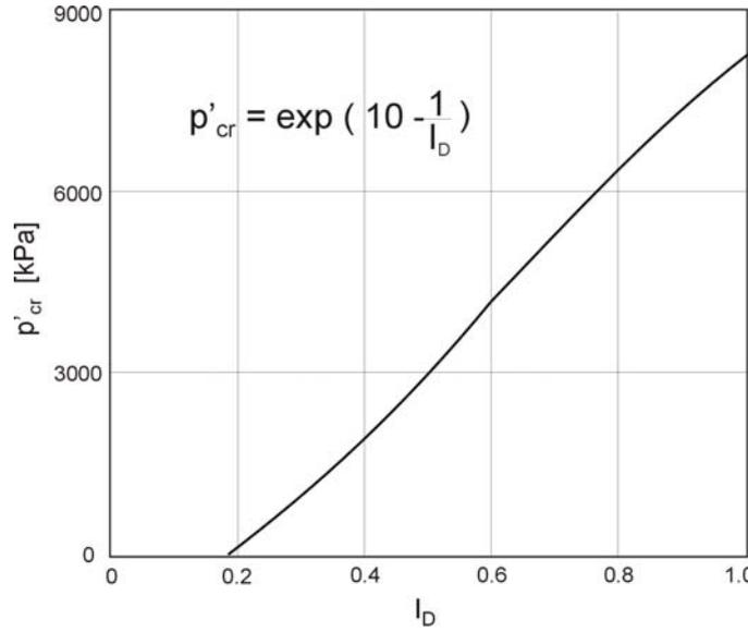
Fig. 1. The dependence  $p'_{cr}$  on  $I_D$  for silica sand
