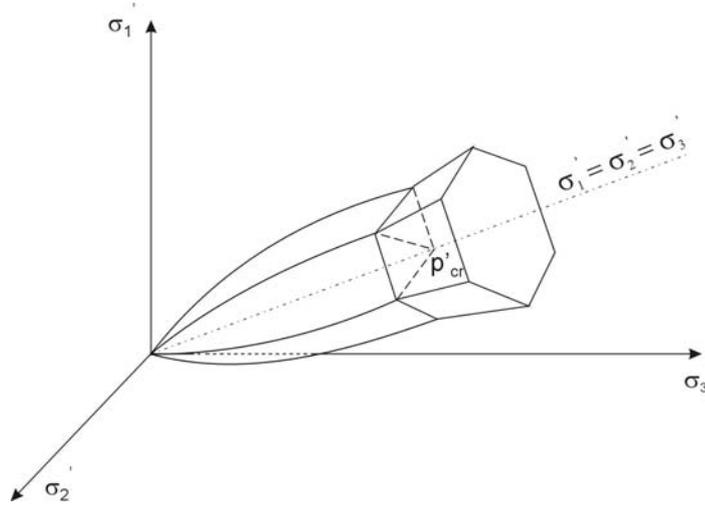
Fig. 3. The non-linear Mohr–Coulomb criterion in principal stress space
