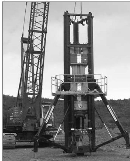
Fig. 5. STATNOMIC load capacity testing equipment
