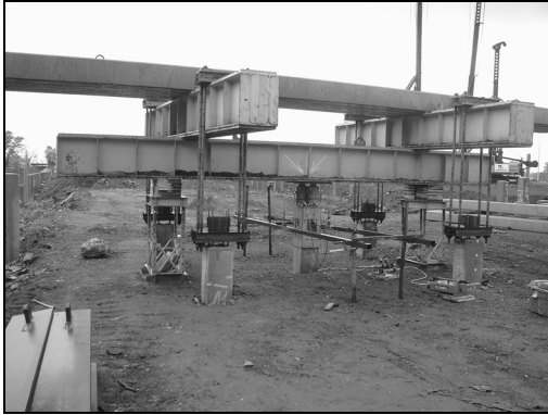
Fig. 1. Static load testing stand
