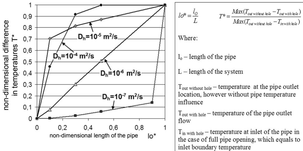
Fig. 11. Extracted, non-dimensional differences in pipe outlet flow temperatures versus non-dimensional pipe length. Unsteady-state modelizations. System length, 1 m; height, 1 m. Pipe radius, 5 cm. Minimum and maximum step temperatures are, respectively, 5 °C and 25 °C
