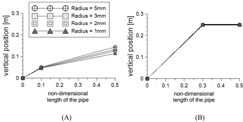
Fig. 10. Variation of vertical position for maximum value point of inlet temperature deficiency in field of extracted thermal influence of pipe versus non-dimensional pipe length. Steady-state modelizations. Inlet and outlet temperatures equal to 25 °C and 5 °C, respectively. Length and height of system, 1 m. Hydraulic diffusivity (defined for system before pipe appearance): (A)  $10^{-5} \text{ m}^2/\text{s}$ , (B)  $10^{-6} \text{ m}^2/\text{s}$
