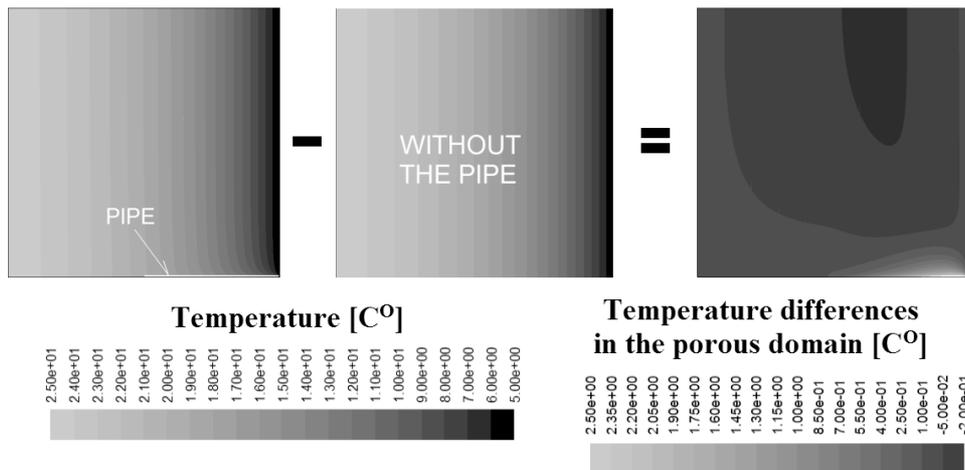
Fig. 4. Scheme of pipe thermal influence extracting
