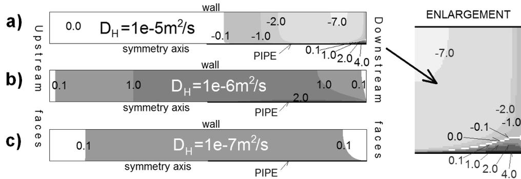
Fig. 7. Extracted thermal influence of pipe at different hydraulic diffusivity values (defined for system before pipe appearance) for steady-state modelizations. System length, 10 m; height, 1 m. Pipe radius, 1 cm; pipe length, 0.5 m. Inlet and outlet temperatures equal to 25 °C and 5 °C, respectively
