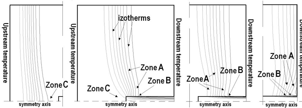
Fig. 5. Example of thermal front passage through highly diffusive porous domain (hydraulic diffusivity of  $10^{-4} \text{ m}^2/\text{s}$  defined for system before pipe appearance). Pipe length, 500 mm; pipe radius, 50 mm; length and height of system, 1000 mm
