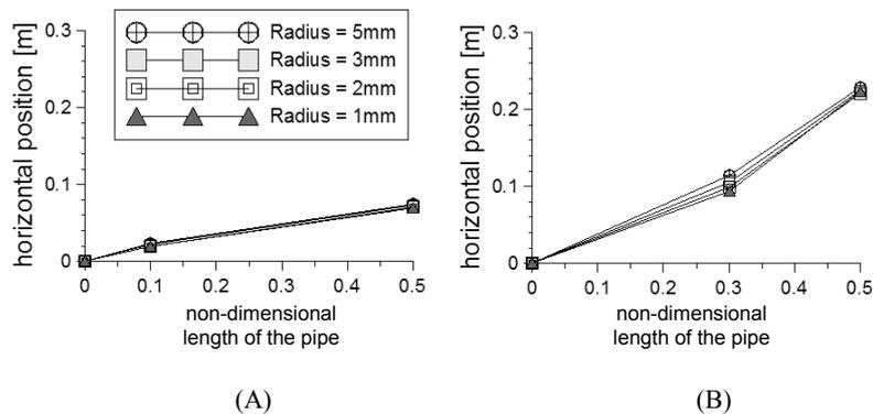
Fig. 9. Variation of horizontal position of point of maximum values of inlet temperature deficiency in field of extracted thermal influence of pipe versus non-dimensional pipe length. Steady-state modelizations. Inlet and outlet temperatures equal to  $25^\circ\text{C}$  and  $5^\circ\text{C}$ , respectively. Length and height of system, 1 m. Hydraulic diffusivity (defined for system before pipe appearance): (A)  $10^{-5} \text{ m}^2/\text{s}$ , (B)  $10^{-6} \text{ m}^2/\text{s}$
