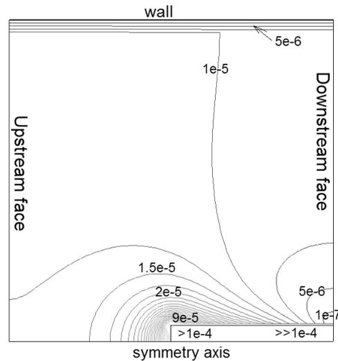
Fig. 6. Example of scalar water velocity field (m/s) in porous zone, evoked by pipe presence.
