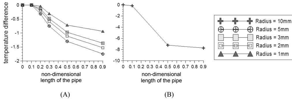
Fig. 8. Maximum values of inlet temperature deficiency in field of extracted thermal influence of pipe versus non-dimensional pipe length. Steady-state modelizations. Hydraulic diffusivity,  $10^{-5} \text{ m}^2/\text{s}$  (defined for system before pipe appearance). Inlet and outlet temperatures equal to  $25^\circ\text{C}$  and  $5^\circ\text{C}$ , respectively. Length of the system: (A) 1 m, (B) 10 m
