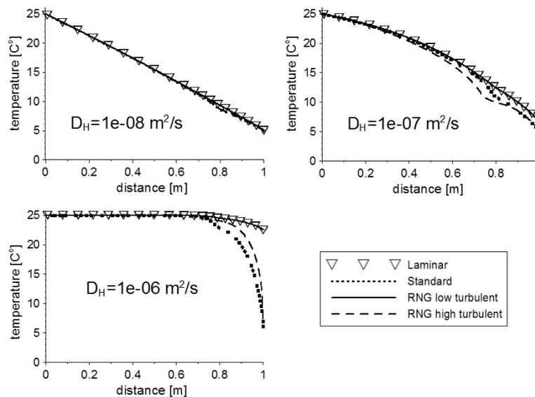
Fig. 3. Comparison of pipe water flow models. Temperature measured in axis of system. Cylinder length, 1 m; pipe length, 0.2 m; pipe radius, 2 mm. Inlet and outlet temperatures of 25 °C and 5 °C, respectively. Hydraulic diffusivity ( $\text{m}^2/\text{s}$ ) defined for system without pipe. Steady-state modelizations
