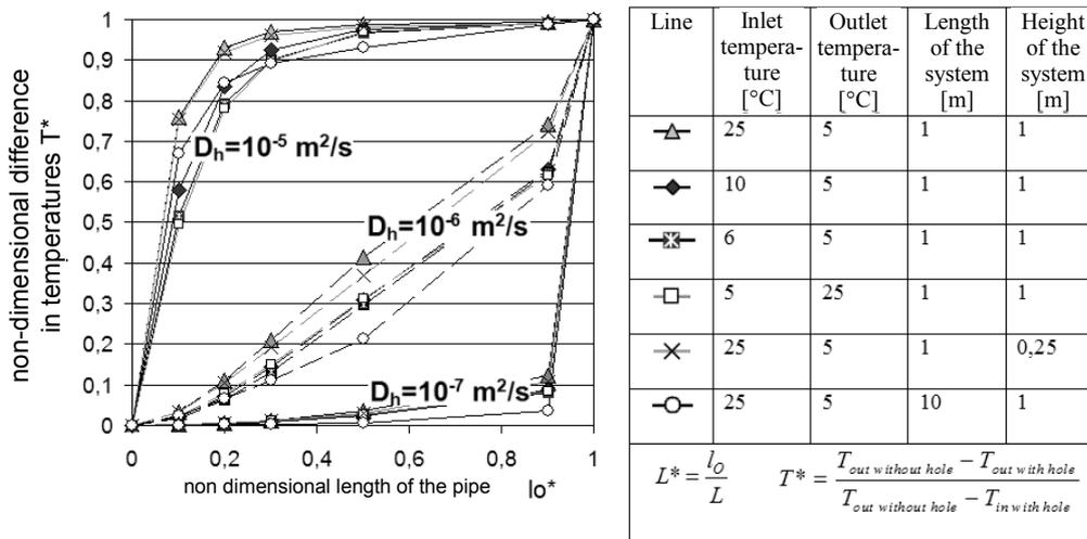
Fig. 12. Extracted, non-dimensional differences in pipe outlet flow temperatures versus non-dimensional pipe length. Steady-state modelizations. Pipe radius, 5 cm
