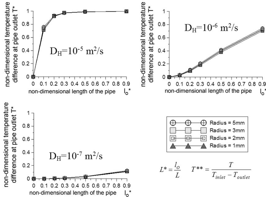
Fig. 13. Extracted, non-dimensional temperature differences in pipe outlet flow versus non-dimensional pipe length at different radii of pipe. Steady-state modelizations. Inlet and outlet temperatures equal to 25 °C and 5 °C, respectively. Length of system, 1 m
