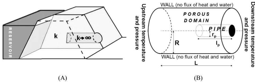
Fig. 2. Scheme of cylindrical domain used for coupled heat and water transport modelization: (A) system under consideration, (B) simplified cylindrical 3D model
