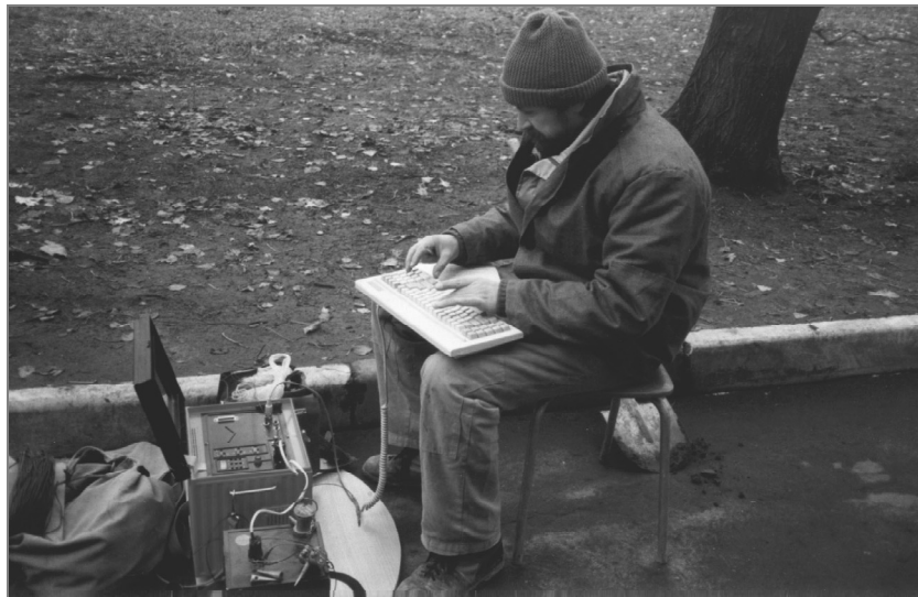
Fig. 2. Procedure of field data acquisition by SRM method
