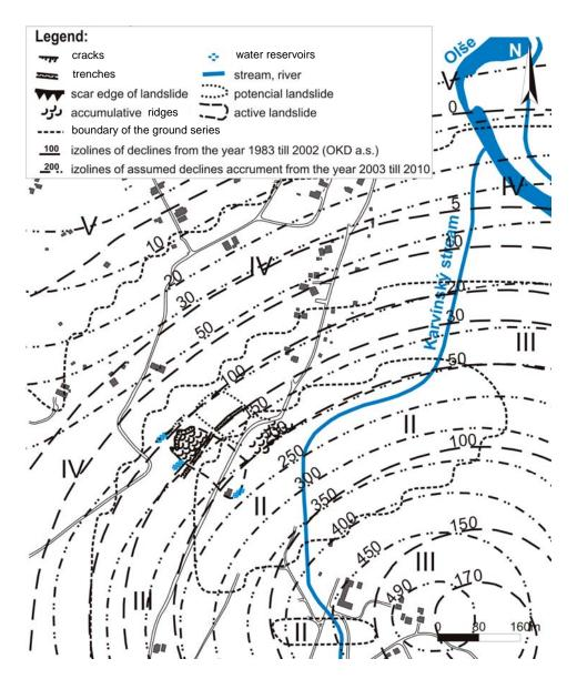
Fig. 2. Declines in centimetres caused by mining in the periods of 1983–2002 and the forecast increase by 2010 with marked positions of slope deformations
