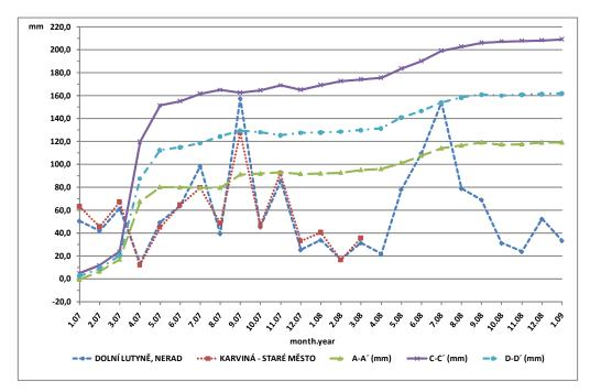
Fig. 4. Chart of measured landslide movements and monthly precipitation from two nearest rainfall gauging stations to the Doubrava Oplíží slope deformation for the monitored period
