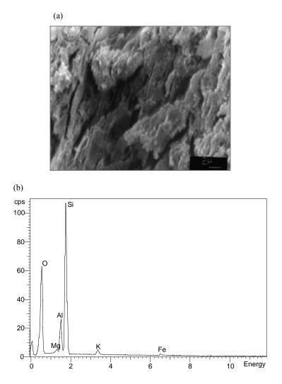
Fig. 6. (a) An example of microstructure surface of clay shales observed in SEM (scale 10000:1), and (b) analysis of their chemical composition with use of X-ray fluorescence (Oxford LINK ISIS-EDS)
