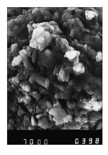
Fig. 3. Microstructural surface of binder taken from laboratory samples of granulated marl eluvium after recrystallization of calcite observed in SEM, scale 4200:1
