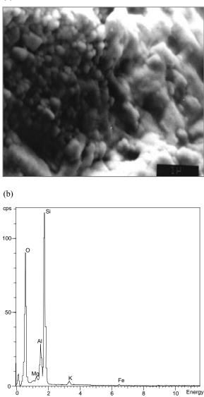
Fig. 5 (a) An example of microstructure surface of weathered clay shales observed in SEM (scale 10000:1), and (b) analysis of their chemical composition with use of X-ray fluorescence (Oxford LINK ISIS-EDS)
