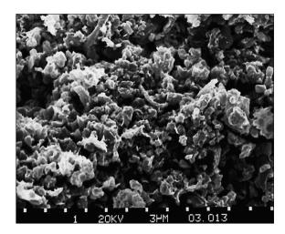
Fig. 2. Microstructural surface of binder of marl eluvium observed in SEM, scale 3000:1
