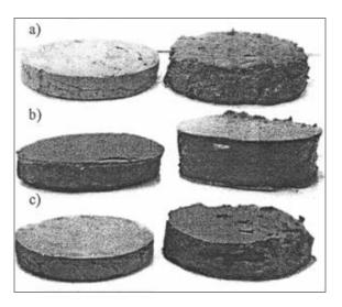
Fig. 7. Examples of soil samples with smectite and illite minerals after the investigation
