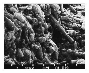
Fig. 1. Microstructural surface of solid chip from marl eluvium observed in SEM, scale 3000:1
