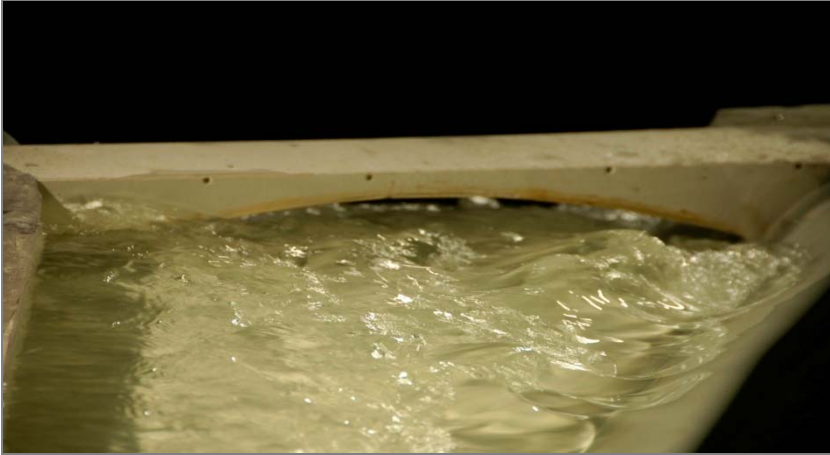
Fig. 12. Road bridge work under conditions of the discharge of about 400 m 3 /s (change III)
