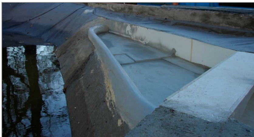
Fig. 6. View of side channel spillway model after change II
