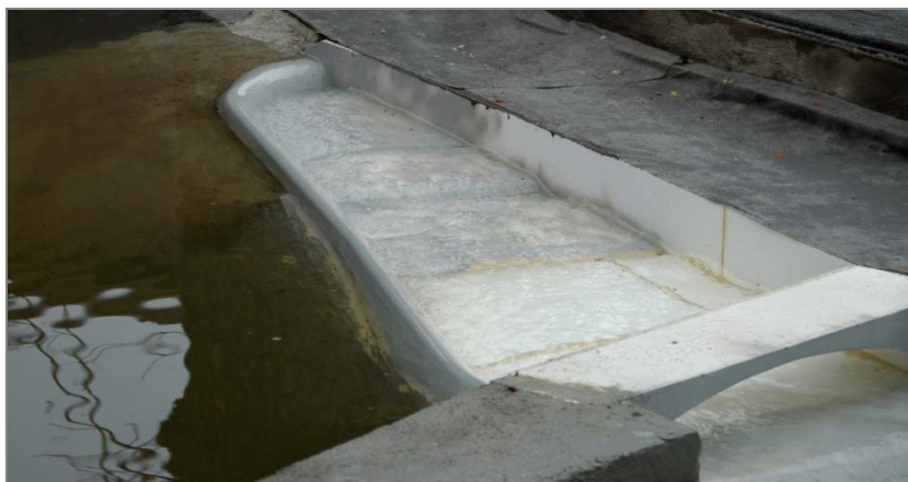
Fig. 5. View of side channel spillway model for existing configuration (change I)
