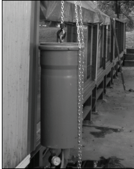
Fig. 3. The tank that provokes seepage flow in the z-direction
