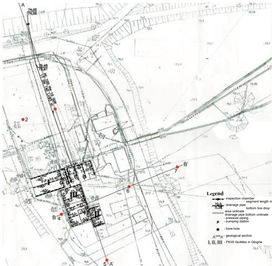
Fig. 6. Draining through raising the cellar floor and performing internal drainage
