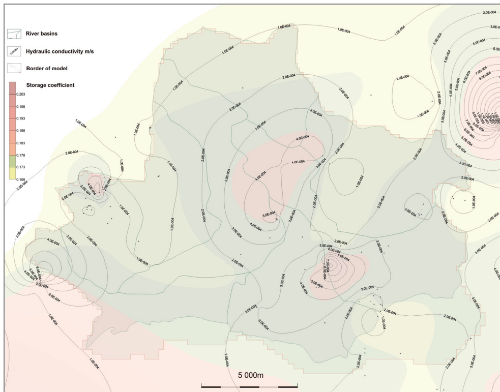
Fig. 5. Distribution of hydraulic conductivity and storativity
