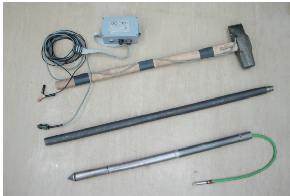
Fig. 1. Measurement equipment of the seismic module with single tri-axial accelerometer set
