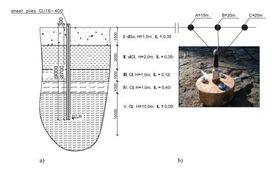
Fig. 1. General view of field tests site: (a) geotechnical profile with selected soil parameters, (b) picture of the stand and of vibration sensors situated at a distance of 15, 20 and 25 m from the place of sheet piles driving
