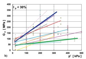
Fig. 7. Shear modulus versus average effective stress in soils under study: (a) for  $I_p > 30\%$ , (b)  $I_p < 30\%$  (Lipiński et al. [9])
