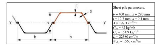
Fig. 2. Sheet pile parameters: A – area,  $G_{so}$  – weight of 1 m of pile,  $G_w$  – weight of 1 m<sup>2</sup> of pile,  $I_y$  – moment of inertia,  $W_{el,y}$  – elastic bending coefficient
