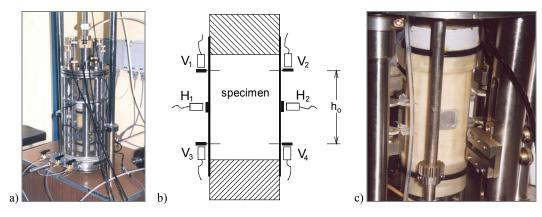
Fig. 5. Test stand: (a) modified chamber of the triaxial apparatus in the Department of Geotechnics, Silesian University of Technology; (b) basic configuration of six sensors system for micro-strains measurements, (c) specimen with six local sensors mounted
