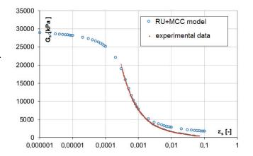
Fig. 8. Typical RU+MCC relationship of "G– $\varepsilon_s$ " vs. experimental triaxial test data
