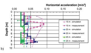
Fig. 11. Comparison of analyses results with field tests results: (a) vertical accelerations amplitudes, (b) horizontal acceleration amplitudes
