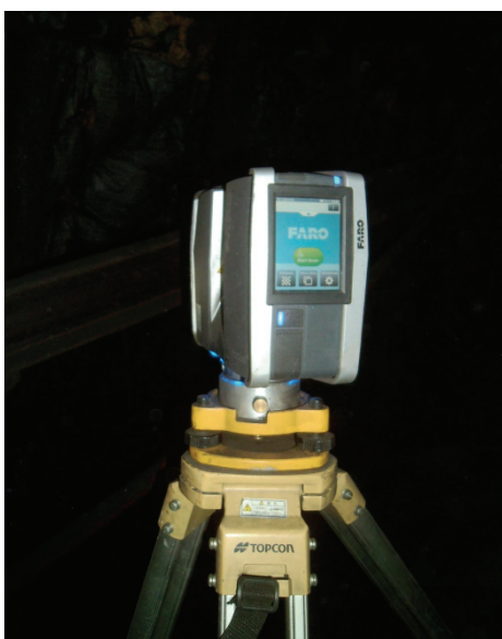
Fig. 3. The FARO Focus 3D scanner during operation
