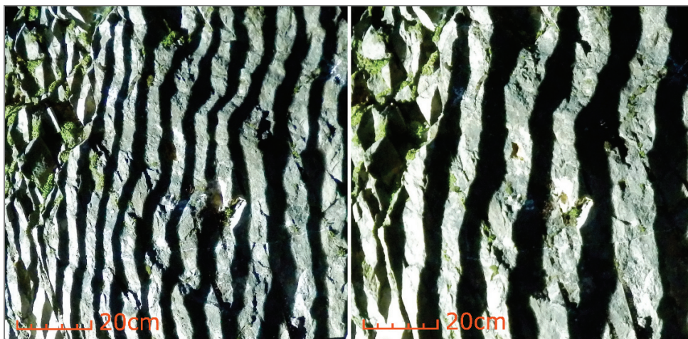
Fig. 3. Curved bit planes on measured rock surface. On the left, 16px bit plane. On the right, 32px bit plane
