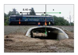
Fig. 7. Loading soil-steel structure with locomotive
