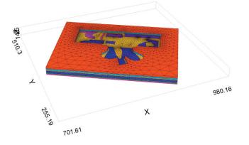
Fig. 4b. Spatial image of the numerical model used to predic settlement of soils and foundation slab deformations
