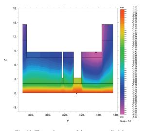
Fig. 15. The settlements of the system soil-slab in the cross-section B1-B1'. (Settlements are expressed in meters; scale multiplier = 1e-2)
