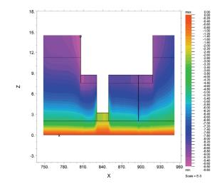
Fig. 14. The settlements of the system soil-slab in the cross-section A1-A1'. (Settlements are expressed in meters; scale multiplier = 1e-3)
