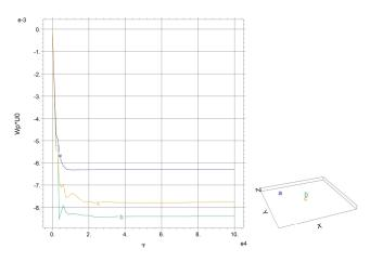
Fig. 16. The settlement of the top surface of the slab at three chosen points in time. (Settlements are expressed in meters; scale multiplier = 1e-3)
