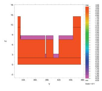
Fig. 8. Plastic potential in the cross-section B1-B1' according to the Drucker–Prager criterion
