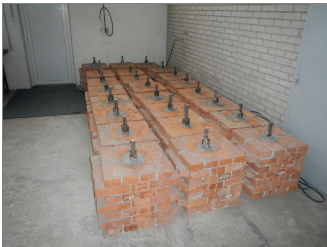
Photo 10. Test specimens modelling brick foundations
