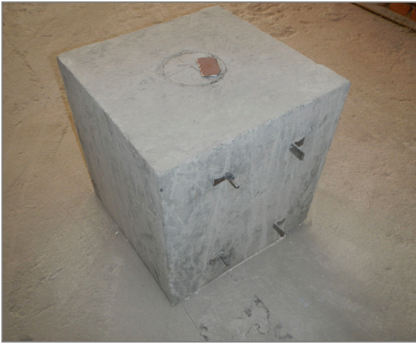
Photo 3. Specimen modelling foundation made of concrete
