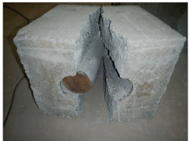
Photo 9. Pile after concrete specimen failure
