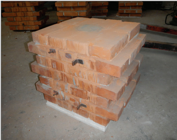
Photo 4. Specimen modelling foundation made from brick
