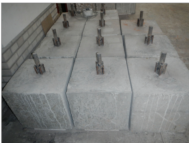
Photo 11. Test specimens modelling concrete foundations
