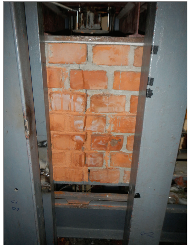
Photo 12a. Final fracture of brick foundation specimen
