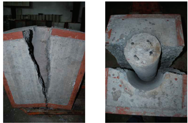
Photo 2. Form of specimens failure
