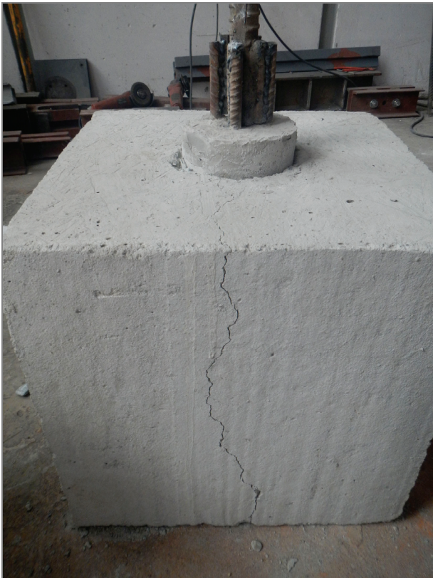
Photo 13. Concrete foundation specimen after the test
