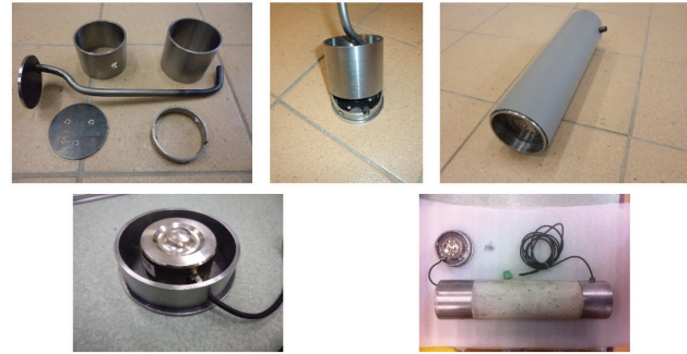
Figure 1: Components of instrumentation pile model.
