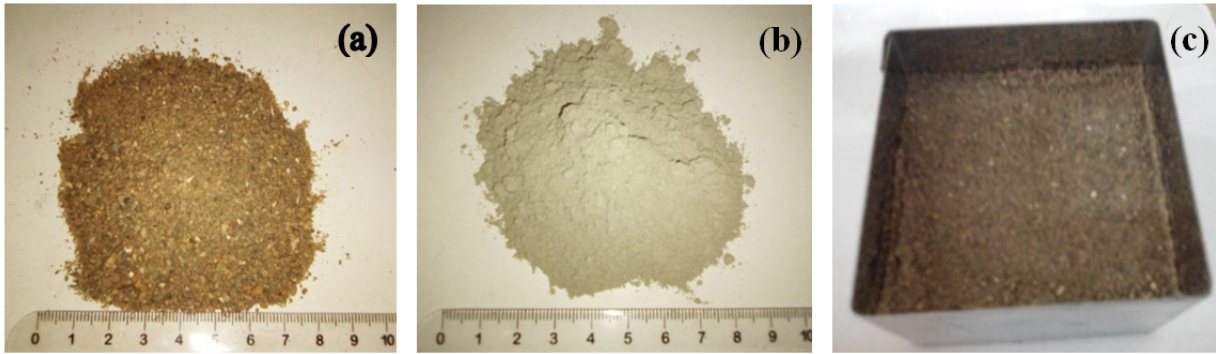
Figure 3: Materials used in this study: (a) Sand, (b) Cement, (c) Sample preparation.
