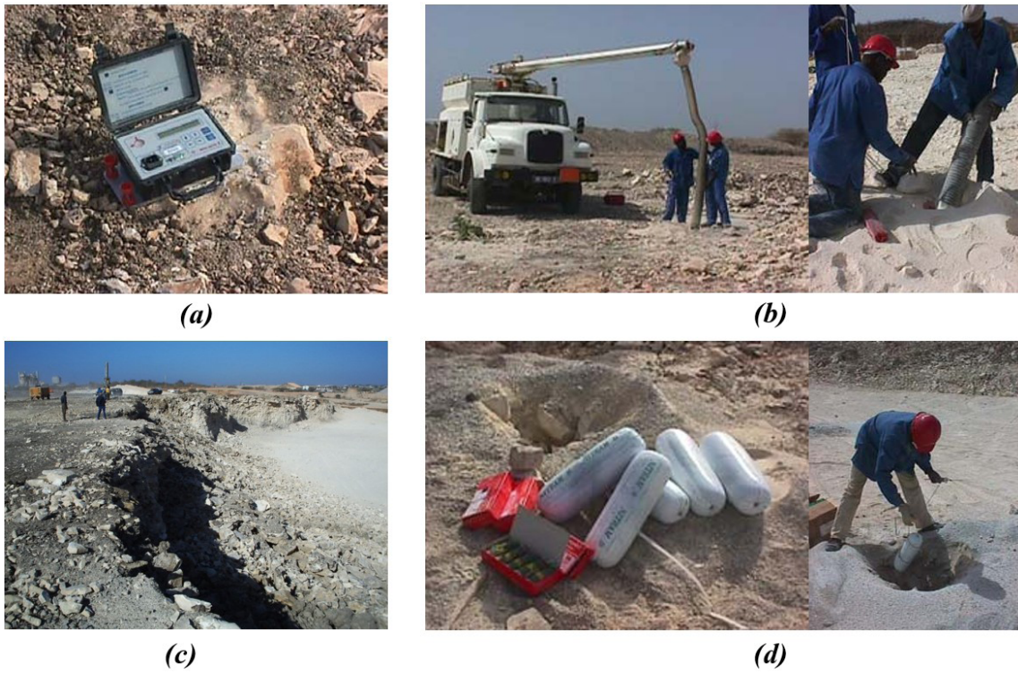
Figure 2: (a) Vibration monitoring sensor; (b) ANFO truck loader; (c) Blast area inspection; (d) Bottom charge with cartridges and electric detonators.
