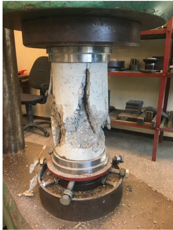
Figure 6: Failed concrete specimen.
