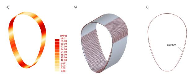
**Figure 5:** Stress distribution and deformations of the panel when the heat of hydration is equal to 40°C: (a) stress distribution, (b) 3D view of panel deformation, (c) 2D view of panel deformation with an indication of the location where the maximum value occurred.
