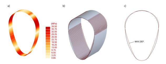
Figure 6: Stress distribution and deformations of the panel when the heat of hydration is equal to 50°C: (a) stress distribution, (b) 3D view of panel deformation, (c) 2D view of panel deformation with an indication of the location where the maximum value occurred.
