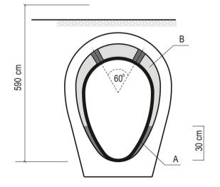
Figure 8: Scheme presenting the distribution of grout in two stages: A – first stage, B – second stage.
