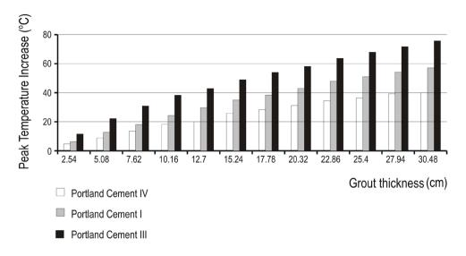
Figure 1: The increase in peak temperature at the casing-grout boundary as a function of grout thickness for three different types of Portland cement grout [16].
