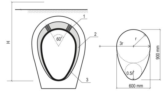
Figure 3: Assembly scheme and geometric characteristics of GRP panels: 1 – wooden spacer, 2 – grout, 3 – brick sewer, H – height from which the grout is distributed.
