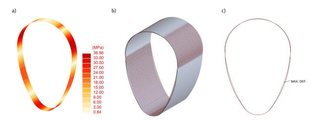
**Figure 4:** Stress distribution and deformations of the panel when the heat of hydration is equal to 25°C: (a) stress distribution, (b) 3D view of panel deformation, (c) 2D view of panel deformation with an indication of the location where the maximum value occurred.
