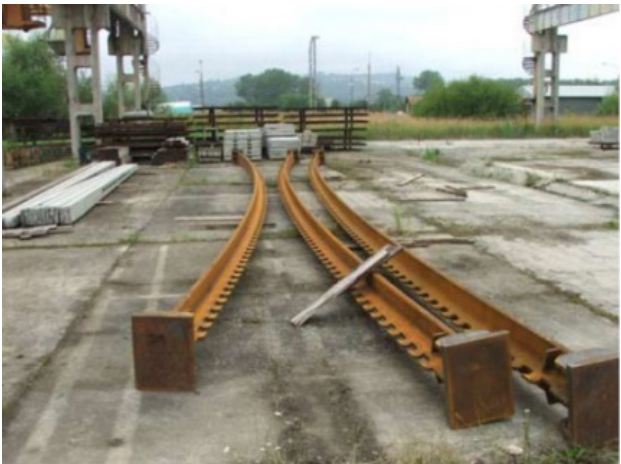
Figure 7: Steel part (“external reinforcement”) of the girders for the pedestrian bridge in Przemyśl, Poland (picture from the proposal of the PreCo-Beam project [7]).
