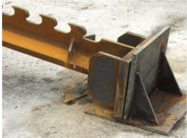
Figure 8: Steel dowels (SA shape according to [7]) used in the girders for the pedestrian bridge in Przemyśl, Poland (picture from the proposal of the PreCo-Beam project [7]).
