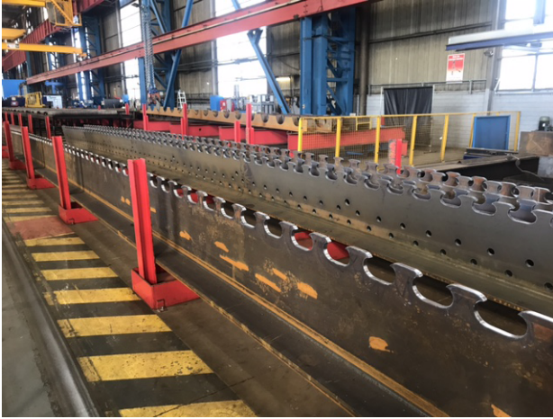
Figure 10: Steel T-sections produced in Luxembourg (picture: ArcelorMittal).
