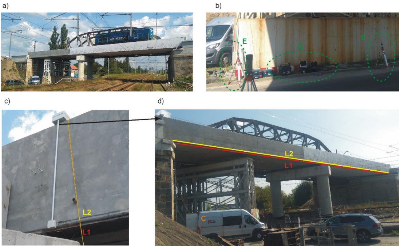
Figure 32: General view of the structure during test. L1 – light wire on steel flange, L2 – light wire on concrete web, E – measuring equipment under the bridge (displacements), C – car with computer for computing light wire recordings.
