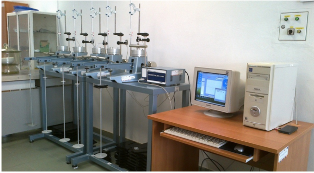
Figure 2: Set of oedometers used for the tests.
